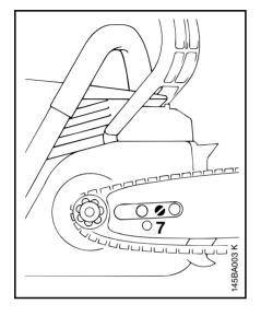
Now turn tensioning screw (7) clockwise until there is very little chain sag on the underside of the bar -
