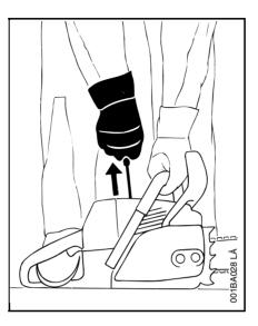
With the **first method**, the chainsaw is started on the ground. Make sure the chain brake is engaged (see "Chain Brake" chapter in your Owner's Manual) and place the chainsaw on firm ground or other solid surface in an open area. Maintain good balance and secure footing.
