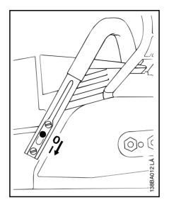
Switching on electric handle heating\*
