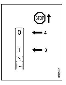
In the "Warm Start" position, continue cranking after engine begins to fire. As soon as the engine runs, **immediately** blip the throttle trigger so that the Master Control lever moves to "Run" idling position -
