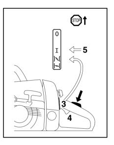
When engine begins to fire: Move Master Control lever (3) to )\( and continue cranking as soon as engine runs, immediately blip the throttle trigger (4) the Master Control lever (3) will move to "Run" position (5) I and the engine settles down to idling speed.
