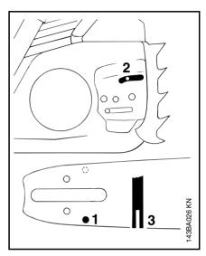
Turn the bar over - every time you sharpen the chain - and every time you replace the chain this avoids one-sided wear, especially at nose and underside of the bar.
