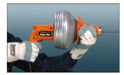
5. Gently squeeze the trigger and move the machine toward the drain opening. *DO NOT FORCE THE CABLE.* The job won't go any faster and you could kink the cable.
